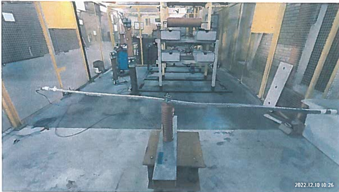
Figure 2: Equipment under dry power frequency and impulse withstand voltage test
