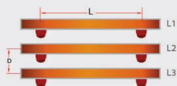
\*  $L_{max}$  : Maximum distance between busbar support centers
